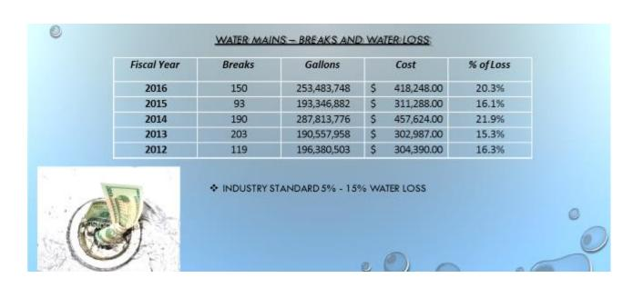
The Public Utilities Department operates and maintains approximately 184.4 miles of water mains. Over one-half of those, 97.4 miles or 514,000 linear feet, are cast iron lines needing to be repaired (lined) or replaced. It is estimated that acoustic monitoring to locate leaks in the water mains would cost approximately \$160,000.00.
